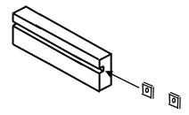
Align the Nuts with the mounting holes in the mount
