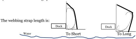
Note: If the dock surface to water height is between 10 and 15 inches, the figure above on the left maybe
