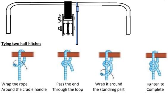
Tying a overhand knot on the loose end will give added security.
