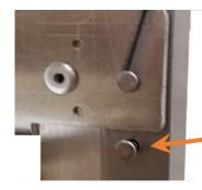
Insert 2<sup>nd</sup> Clevis Pin through hole in bracket and secure with "R" Retaining Clip on opposite side.
